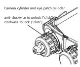
To focus and fine tune eye position use one hand to stabilize the camera cylinder and the other hand to move the camera joystick up/down and side/side until the eye image is central on screen. Firmly pull camera joystick in/out to focus the image of the iris and edge of the pupil. The camera cannot be pushed into the eye as there is an end stop. It is important to focus the eye to ensure that possible torsion is visible.
